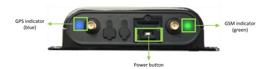
To start the MVT600, press and hold down the power button for 3s to 5s, or connect the MVT600 to external power supply (11 V to 36 V).
