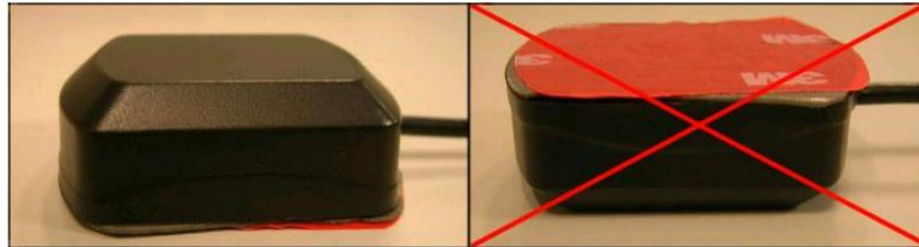
Fig. 3. GPS antenna correct mounting
