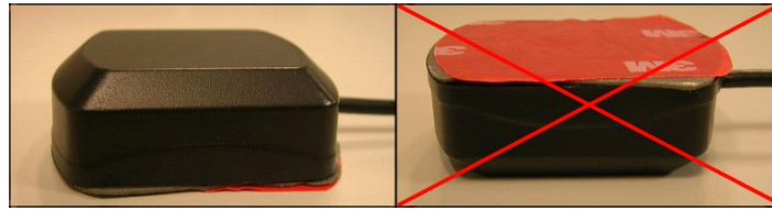
Figure 60 Correct GNSS antenna mounting
